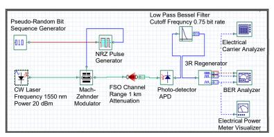
Fig. 2. Block diagram of the simulation setup of the proposed FSO link
