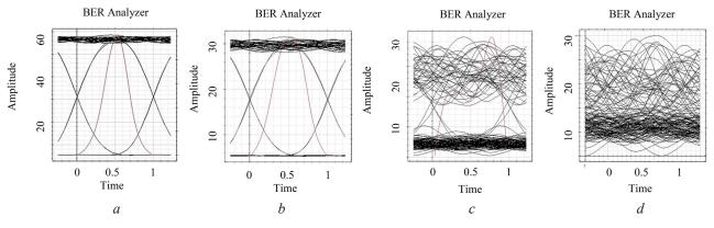
**Fig. 3.** Eye diagram performance of FSO at: a - 0.5 km, 1 mrad; b - 0.5 km, 2 mrad; c - 1 km, 1 mrad; d - 1 km, 2 mrad
