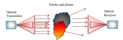
Fig. 1. Block diagram of an FSO system with different divergence angles
