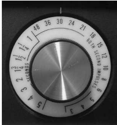
Figure 2-7. Timer dial. Note the increments in impulses ( 1/60 second). (From Langlais RP: Exercises in oral radiology and interpretation, ed 4, Philadelphia, 2004, Saunders.)
