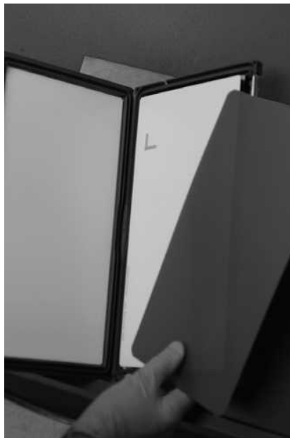
Figure 4-9. Cassette in open position showing front and back intensifying screens and piece of film.
