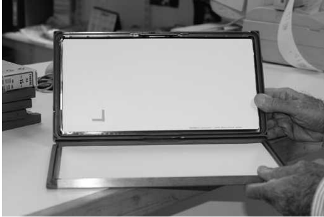
Figure 4-12. | Extraoral cassette left lead marker.
