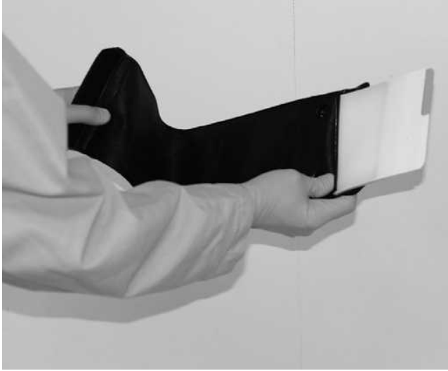
Figure 4-10. Flexible intensifying screen of a panoramic cassette.
