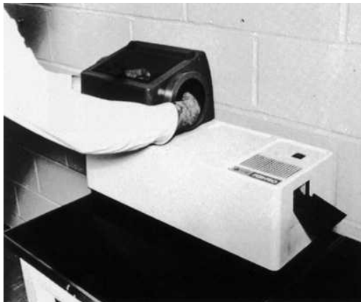
Figure 8-17. Automatic processor with a daylight loader being used in the operatory. Gloves have been removed inside the daylight loader.
