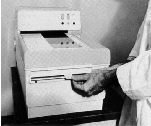
Figure 8-16. Film being inserted into an automatic processor in the darkroom under safelight conditions. Note that gloves have been removed after film was taken from packet.
