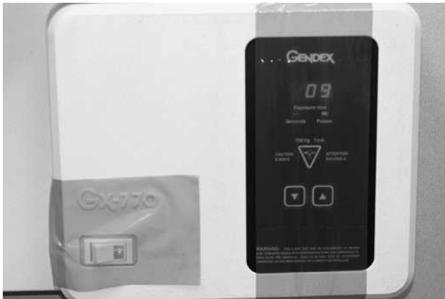
Figure 9-5. | Plastic wrap covering the control panel.
