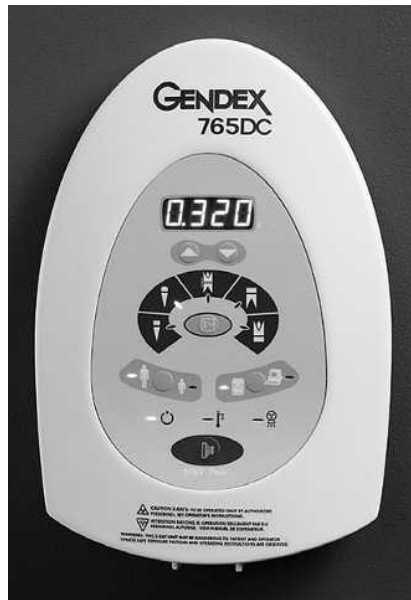
Figure 2-6. Icons on the dental control panel showing size of patient icons. (Courtesy GENDEX Dental Systems, Lake Zurich, IL.)
