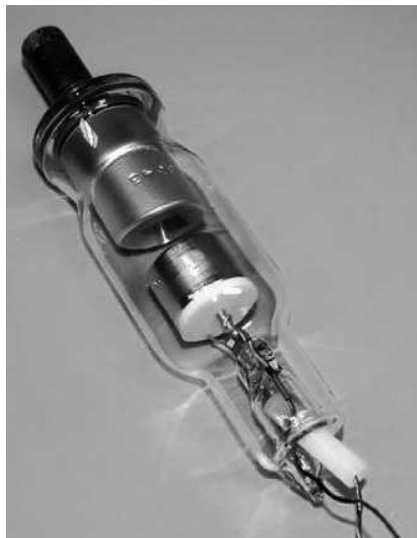
Figure 1-11. | Dental x-ray tube. (Courtesy Xintec, Inc., Research Triangle Park, NC.)
