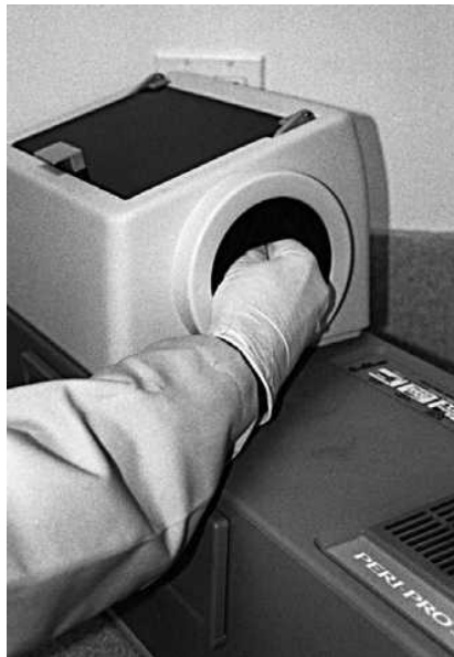
Figure 9-12. The sleeves of an automatic processor have been contaminated by the operator's contaminated gloves.
