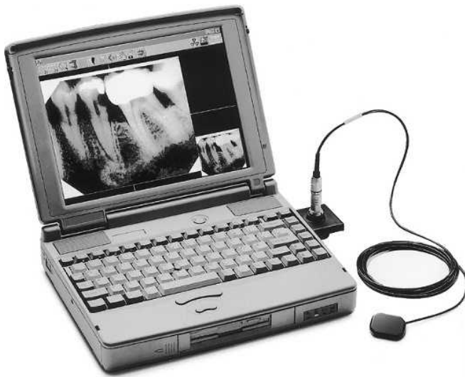
Figure 15-1. A laptop can be used for digital imaging. Note the attached sensor. (Courtesy DEXIS LLC, Atlanta, GA.)
