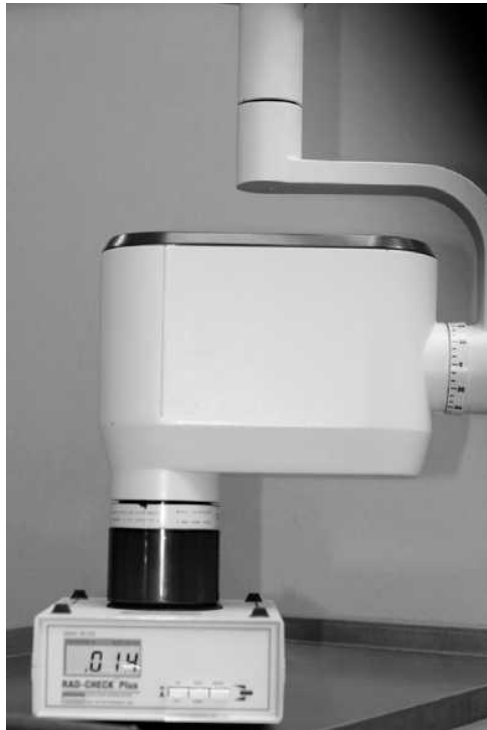
Figure 5-2. | Ionization chamber measuring the output of a dental x-ray machine.
