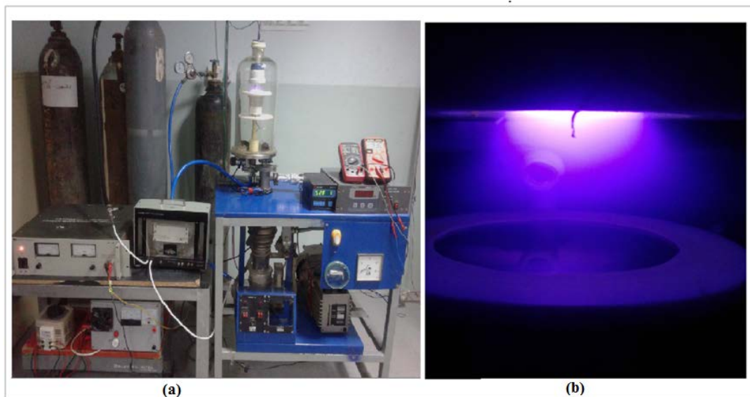
Fig.2:(a) The dc magnetron plasma set-up ,(b) plasma produced between the two electrodes.
