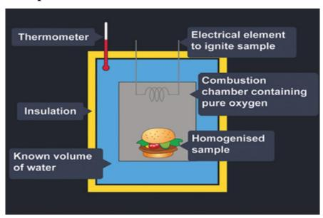
When the food is burned, its caloric value determined by the increase in the temperature of the surroundings water.
